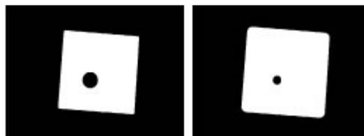
**Figure 37: The effect that is achieved by using an 11 pixels flat disk structuring element.**
